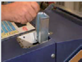
Interchangeable input hoppers for dog tags and medical alert tags for easy change
